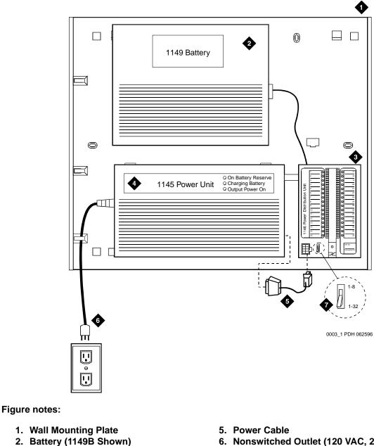
Figure 40: 1145B2/1146B2 Mounting Arrangement
